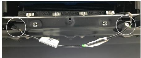
4. With a Standard screwdriver (flathead), bend all the bumper cover mounting clips back to original condiditon. Before picture on left below, after on right.
